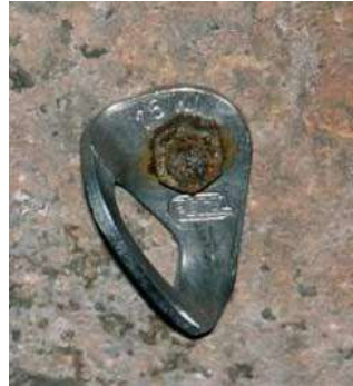
Rusting mild steel expansion bolt. All bolts and hangers should be stainless steel.
