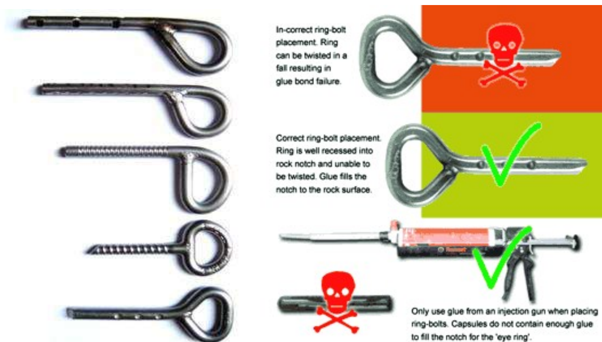
Figure 3a - P Anchor Installation guidelines.
