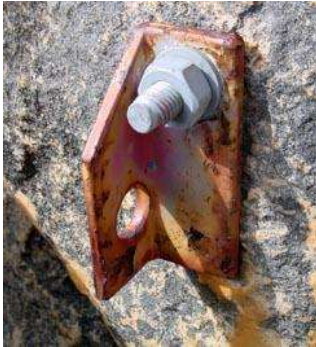
Homemade hanger on mild steel bolt. All bolts and hangers should be stainless steel and hangers should conform with EN-959.
