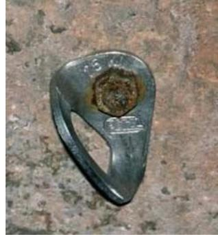
Rusting mild steel expansion bolt. All bolts and hangers should be stainless steel.
