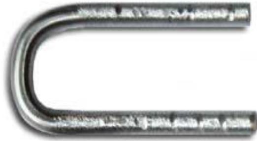
Note the stems are both ground and notched with an angle-grinder
