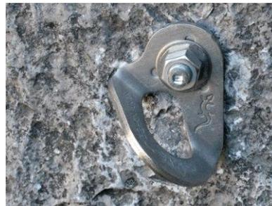
Example of a solid Fixed Anchor safe for use. Rock is solid with no fractures; hanger sits flush with the rock and cannot spin.
